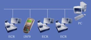
Thanks to its "Power over Ethernet" port, i3070 can be easily connected to an Ethernet LAN, reducing installation and maintenance cost.
